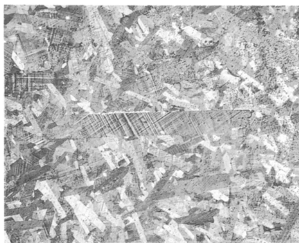
Figure 3 Polarized-light optical micrograph of hot-pressed YBaCuO superconductor before exposure to humidity, showing a high degree of twinning ( \times 423 ).
