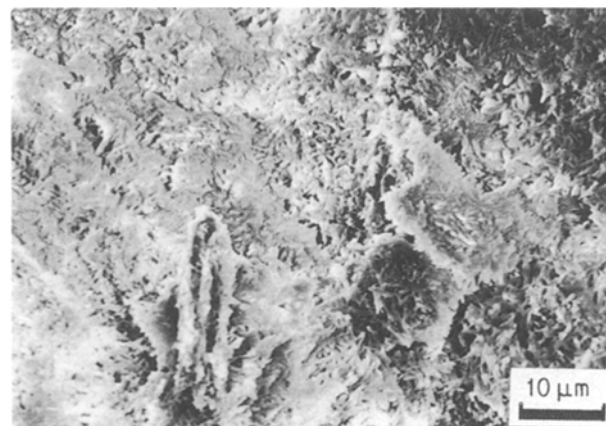
Figure 10 Scanning electron micrograph of hot-pressed sample surface after 840 h exposure, showing the barium precipitates.
